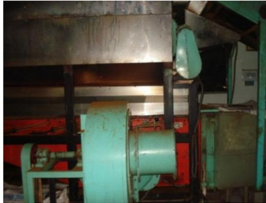
Gambar 2. Vibro Fluid Bed Dryer
